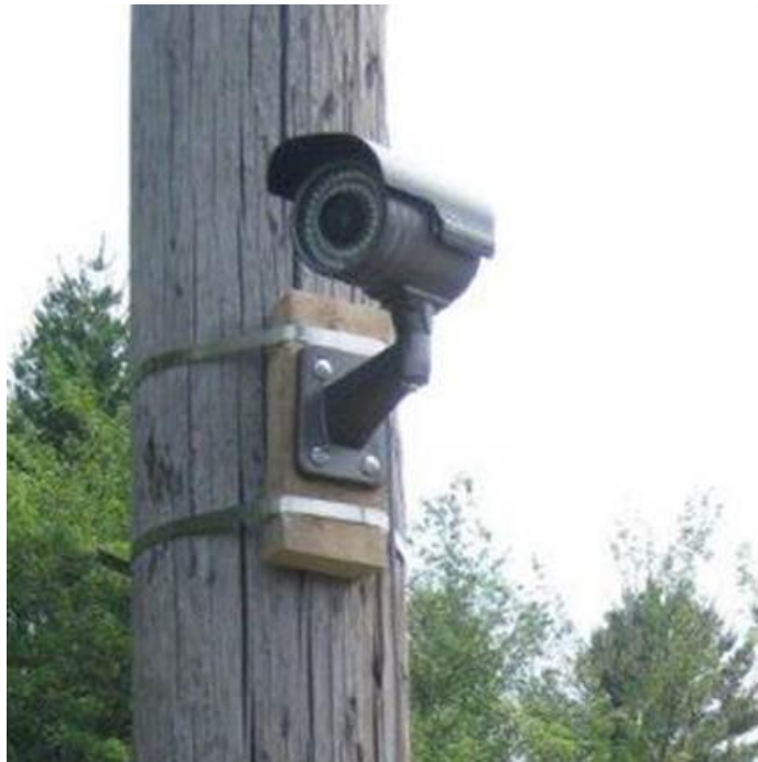
Figure 4 Camera Mounted to Roadside Power Pole
